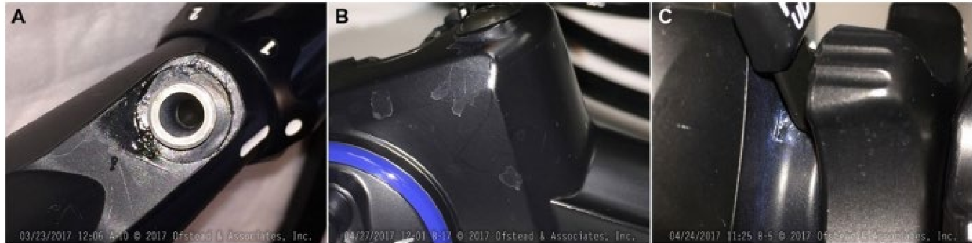
Fig 2. Residues observed on external surfaces of endoscopes. (A) Oily residue near biopsy port of pediatric colonoscope A-10; (B) dried “water spots” on control handle of cystoscope B-17; and (C) whitish-blue, powdery residue under control handle knobs of gastroscope B-5.
